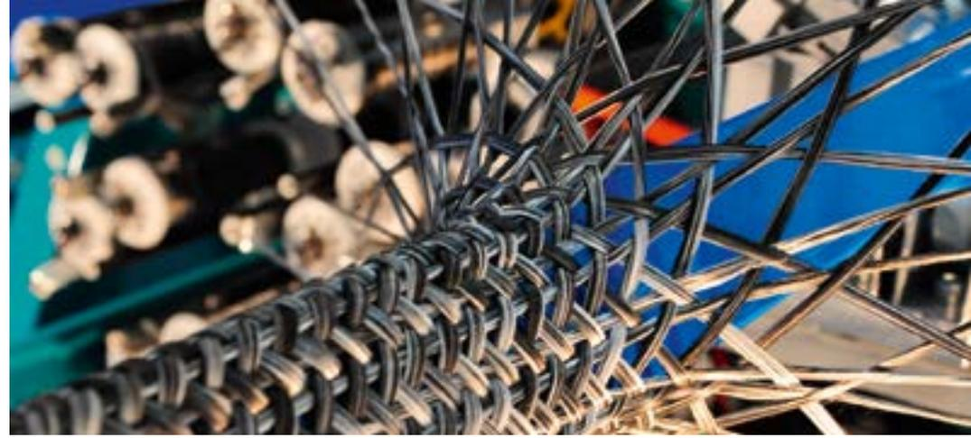
Braiding process for near-net-shape manufacturing of composite fiber structures at the Dresden University of Technology's Institute of Lightweight Engineering and Polymer Technology (ILK).
