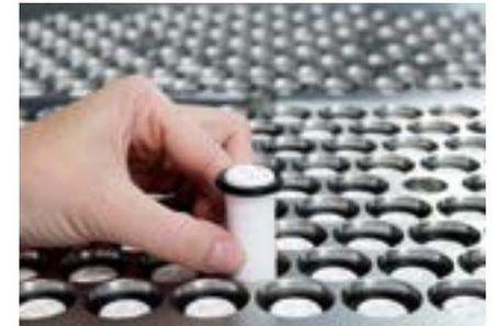
The Fraunhofer IKTS develops nanoporous membranes for energy-efficient separation of bioethanol.
